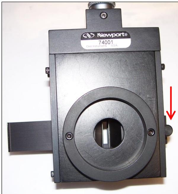
**Figure 13: Tallest Micrometer Adjustable Slit Height.**
